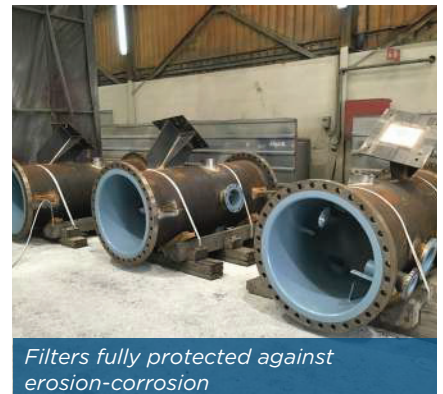
Tank coated with Belzona 5811
