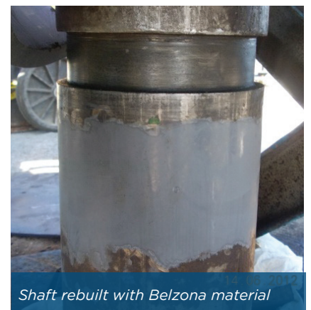
Keyway housing and shaft repaired with Belzona material
