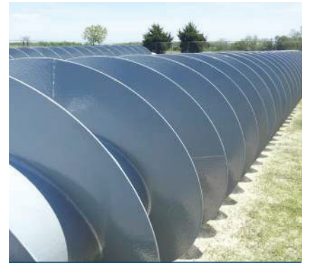
Erosion resistant coating applied
