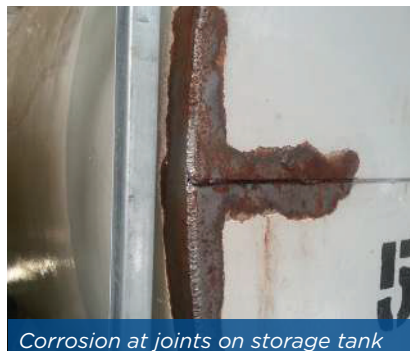
Corrosion at joints on storage tank
