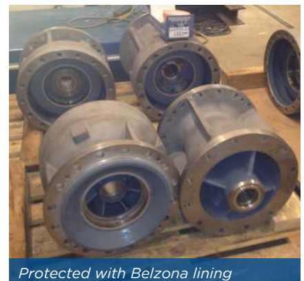
Impeller protected with Belzona lining
