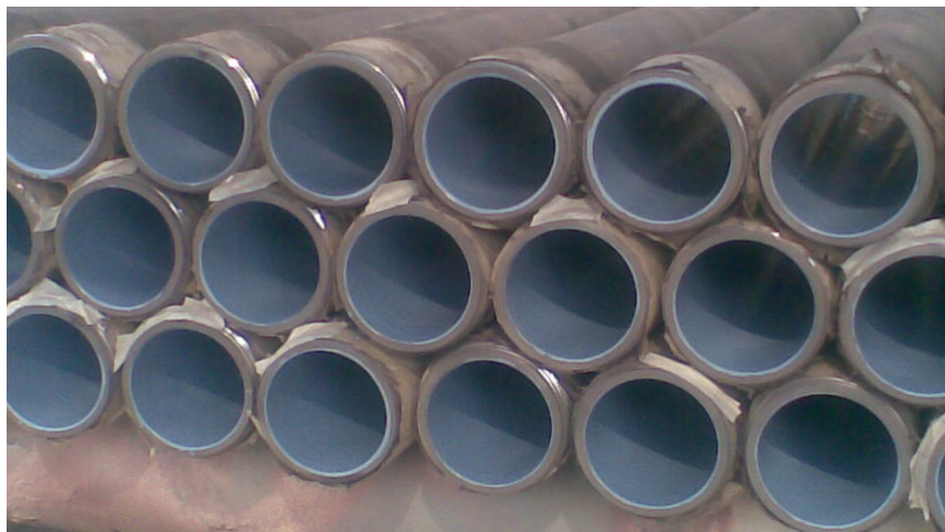
Internal pipe lining
