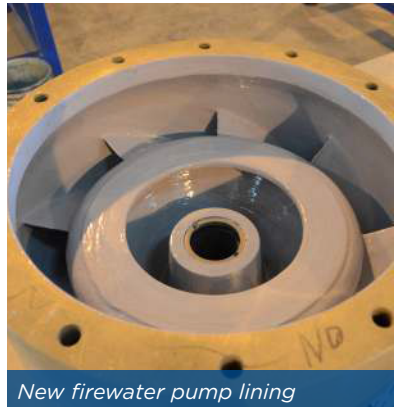
Impeller protected with Belzona lining
