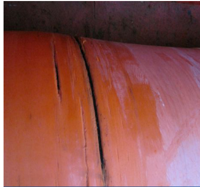
Hose damaged in transport
