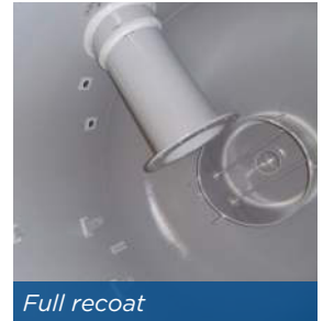
Glass flake lining repair
