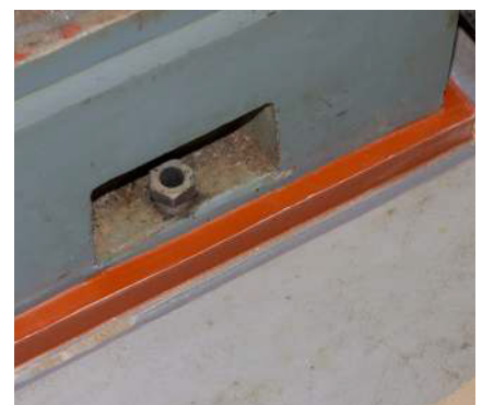
Bespoke chocking solution
