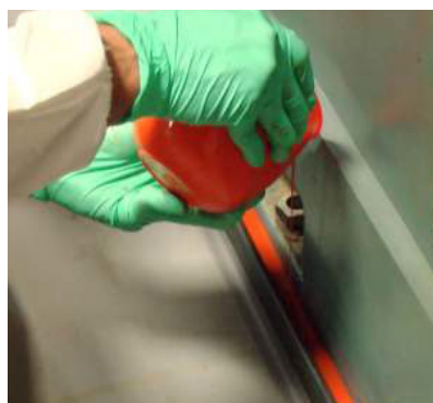
Pourable shimming in action
