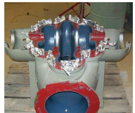
Casing rebuilt and coated
