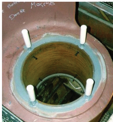
Rudder bearing bonding - top view
