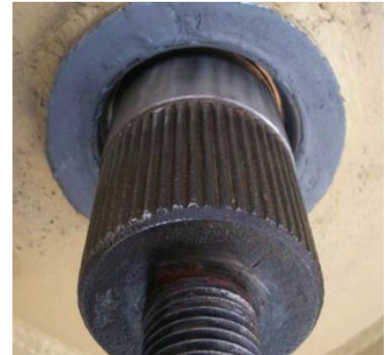
Bearing bushing rebuilt in situ
