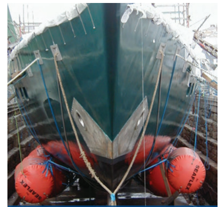
Anchor pocket bonding completed
