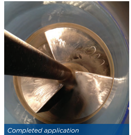
Propeller areas rebuilt and protected
