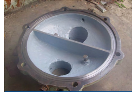
Division bar repaired and protected
