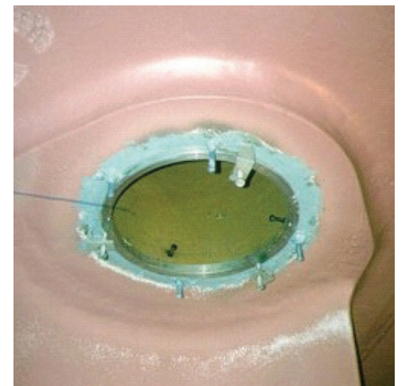
Rudder bearing bonding - bottom view
