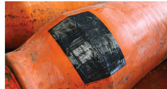
Rubber covers on fuel hoses repaired
