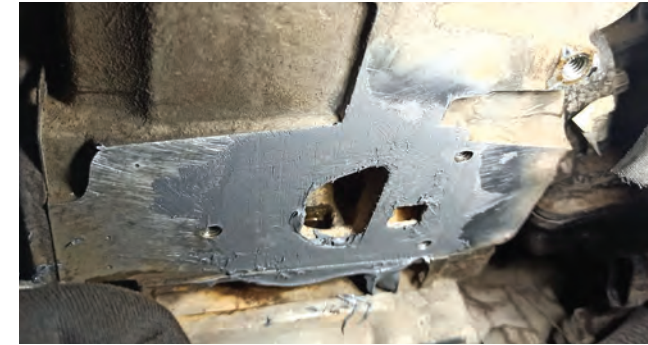
Engine block leaking coolant repaired
