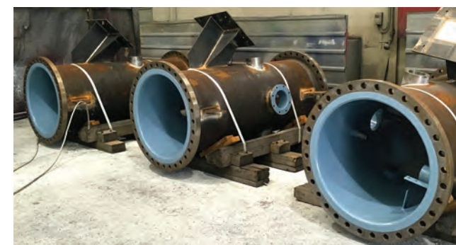
High temperature corrosion protection for new water filters
