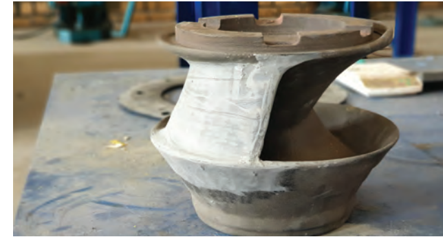
Eroded pump impeller repaired and protected
