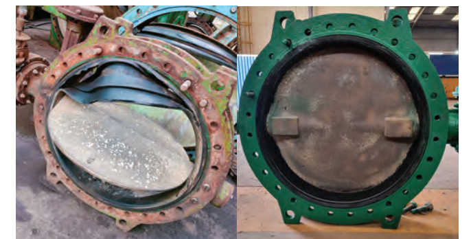
Butterfly valve rubber repaired
