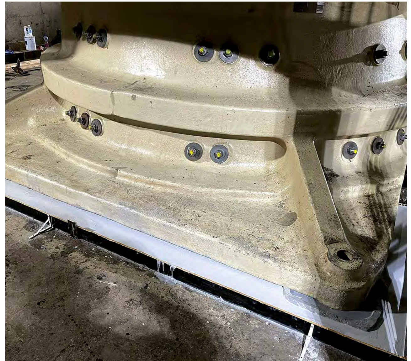
A crusher base stabilized using Belzona anchoring solutions
