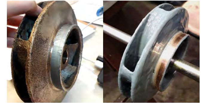
Pump impeller rebuilt and protected from erosion-corrosion
