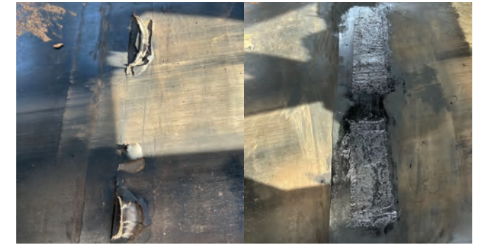
Damaged conveyor belt at a paper mill repaired
