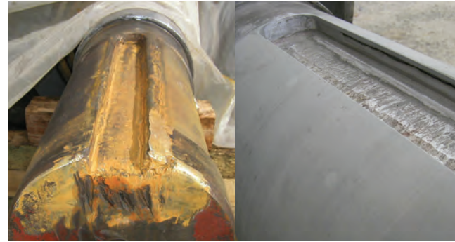
Jaw crusher's damaged shaft and keyway repaired
