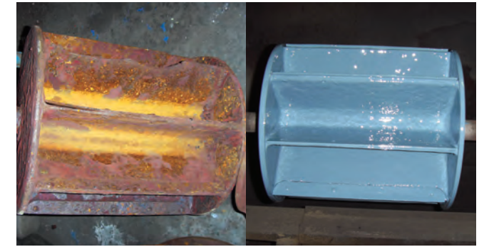
Vacuum pump rotor repaired and protected
